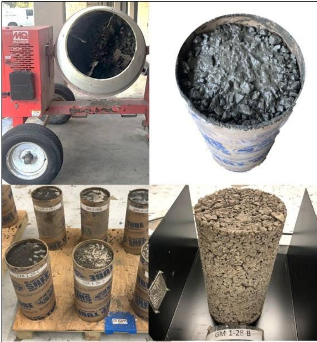
Figure 13-29: Mixing, Casting and Curing Process
