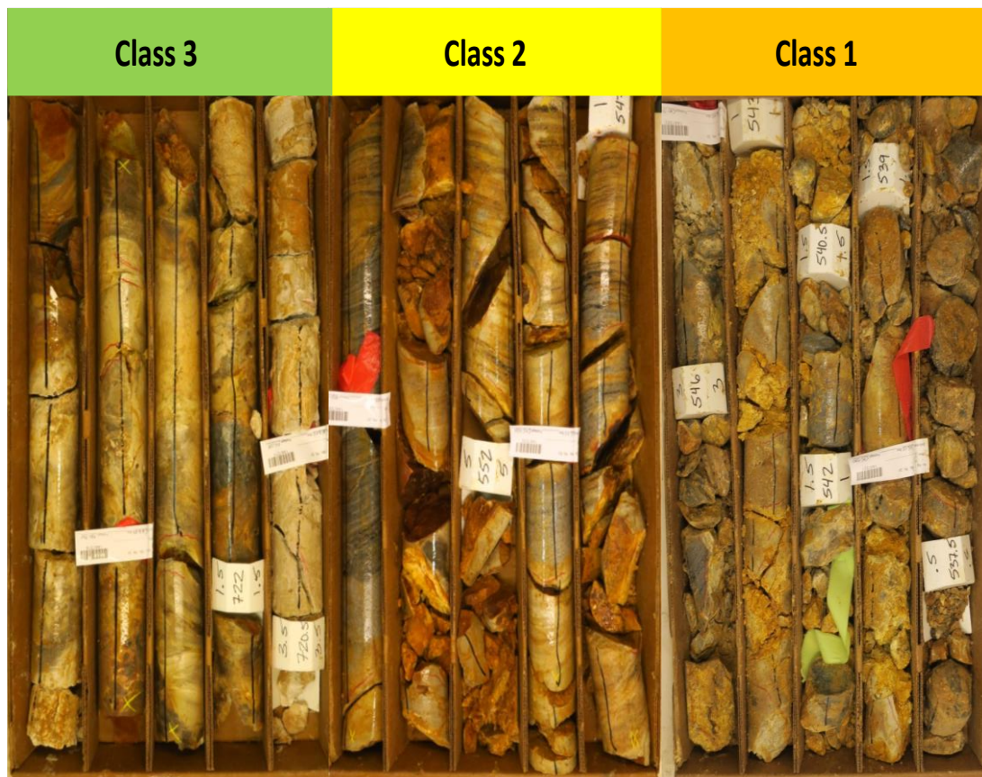
Figure 16.5 Examples of Three Geotechnical Rock Classes
